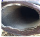
Examples of damage to liner and cement liner
